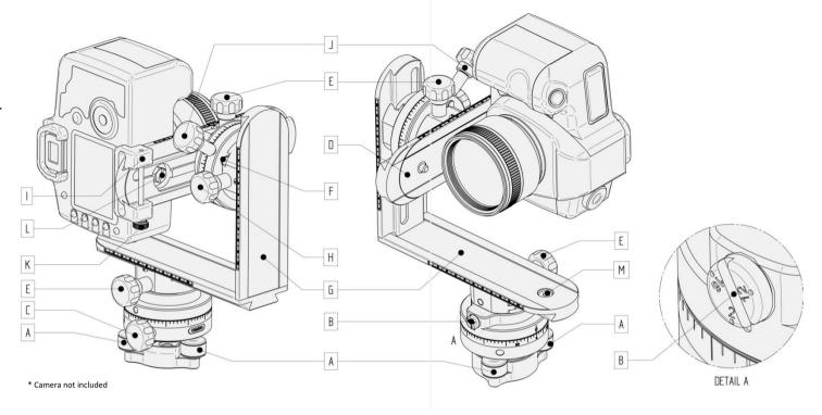
When the relative position of these objects change when turning the panorama head, the sliding plate (D) must be positioned either forwards or backwards until the relative position between these objects is constant. The sliding plate can be locked with knob E. To fully slide the QR-plate from the mount press the release lever (F).
